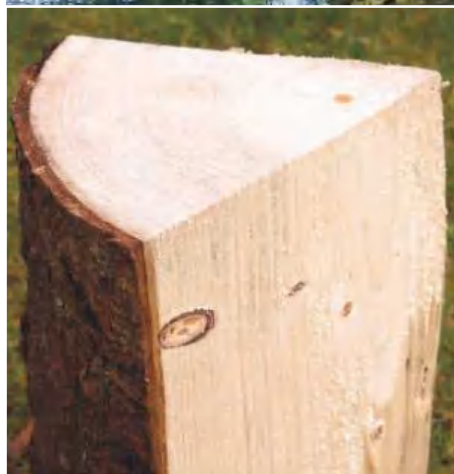
▲ Pic.2 A softwood tree produces a lot of knots from the mass of small branches
